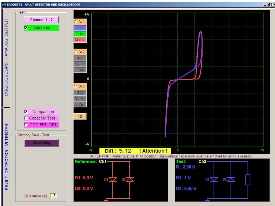
Picture 26: Comparison Test – Parallel Resistor Faults
