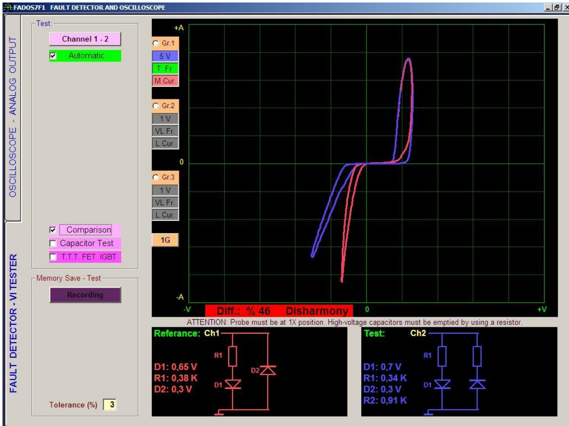
Picture 25: Comparison Test – Integrated Pin Faults
