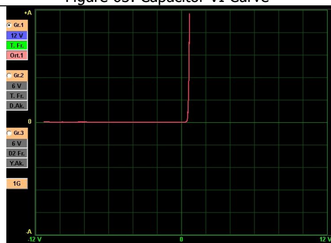
Figure 65: Diode VI Curve
