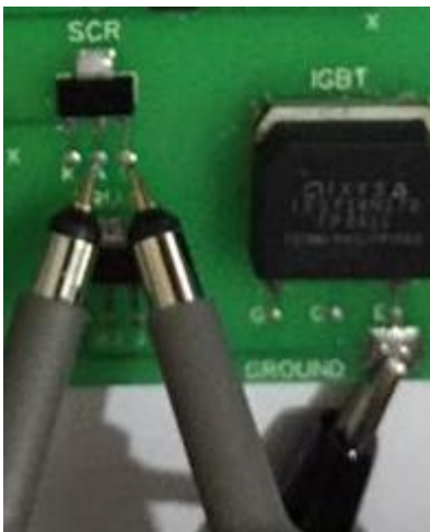
Figure 163: Channel1 (+), Channel2 (+), COM (-) Thyristor Test
