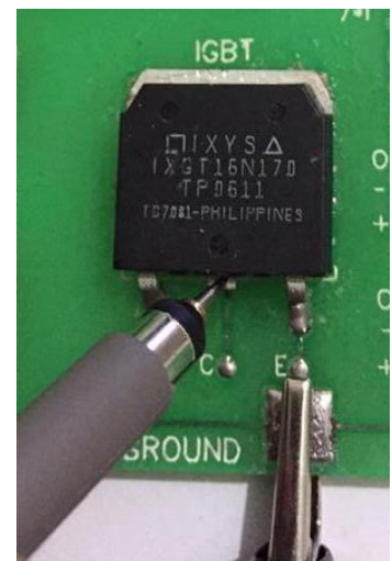
Figure 151: Channel1 Probe Used for Collector - Emitter Measurement
