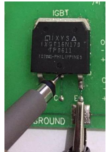
Figure 149: Channel1 Probe Used for Collector - Emitter Measurement
