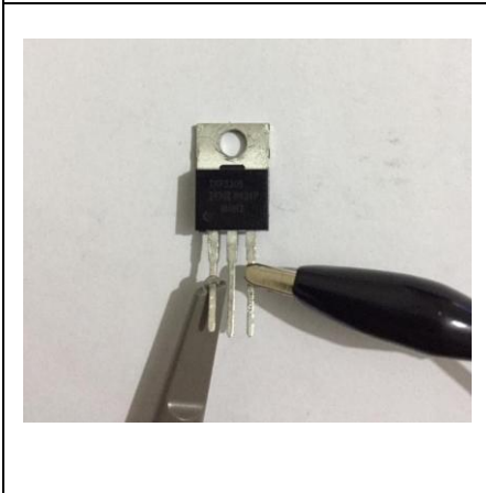
Figure 128: Channel1 Probe Used for Gate - Source Measurement
