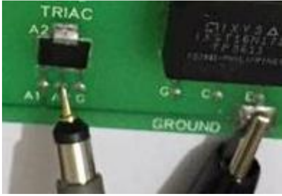
Figure 170: Channel1 Probe Used for Anode2 - Anode1 Measurement
