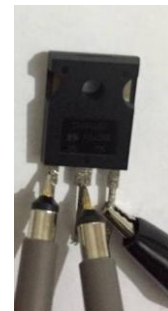
Figure 144: Sample of a Defective N Channel FET
