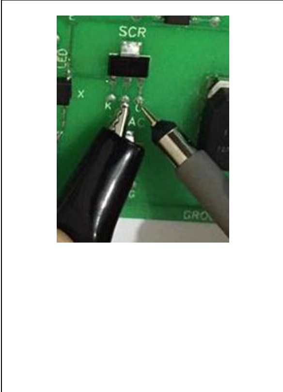
Figure 159: Channel1 Probe Used for Gate - Anode Measurement
