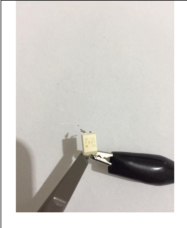
Figure 177: TLP521-1 Test Channel2 (Anode) - COM (Cathode)
